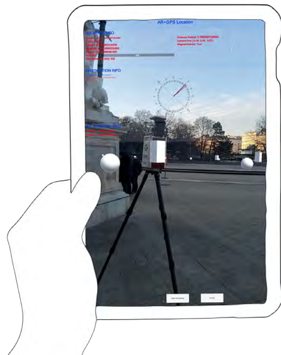
Figure 3 - Screenshot from the AR feedback application; spheres represent photos, boxes represent laserscans - comparison to original laserscanner position visible (by author)
