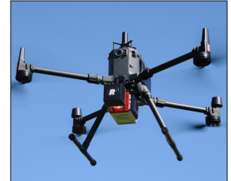
DJI Matrice M300 RTK equipped with RIEGL miniVUX-SYS using RIEGL Integration Kit 300
