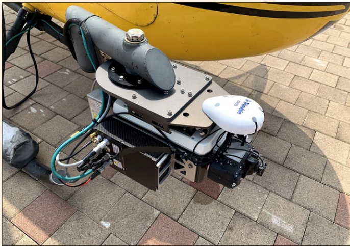
manned helicopter with RIEGL VUX-240 LiDAR Sensor, AP50 Air and nadir RGB camera fully integrated
