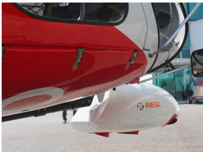
RIEGL's VQX-2 Helicopter Pod mounted to an Airbus Helicopter AS350.
