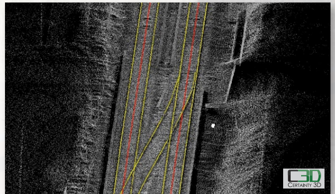
rail specific post processing with various third party software packages possible (shown example data: TopoDOT)
