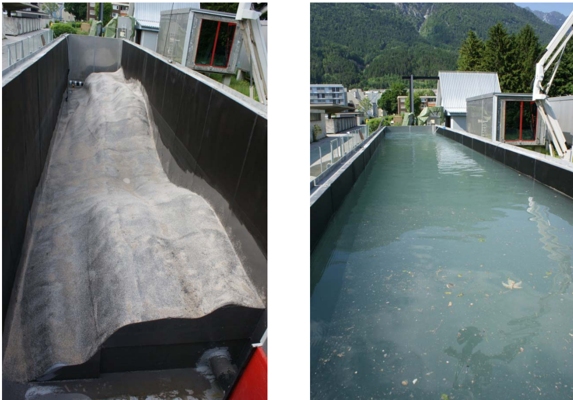
Figure 4: Test site: Empty basin with artificial riverbed (left) and flooded basin with turbid water (right). Basin size 17m x 3m x 2.5m.
