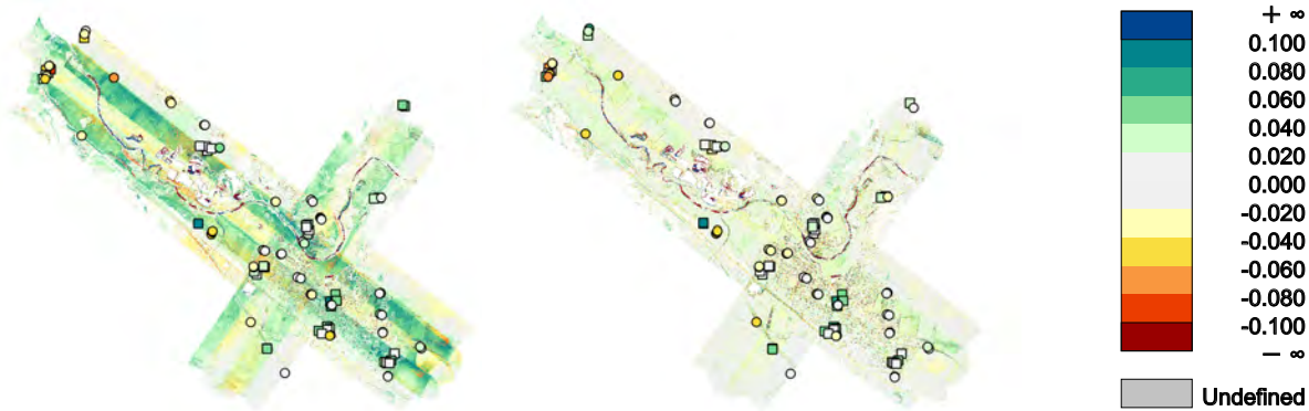
Figure 4. Strip height differences [m] after standard strip adjustment with RiPRECISION (left) and GNSS/INS/LiDAR-integrated adjustment (right). Overlaid on the strip differences are normal distances to ground truth targets of two types: check points on horizontal surfaces on the ground (circles) and on sloped rooftops (squares), after application of the estimated datum shifts.
