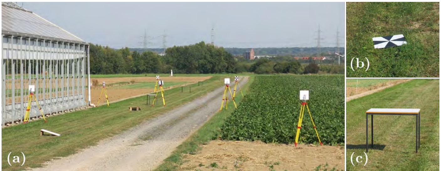
Figure 4. Study area for the analysis of single strip measurement with TLS measurement for the reference point cloud.
