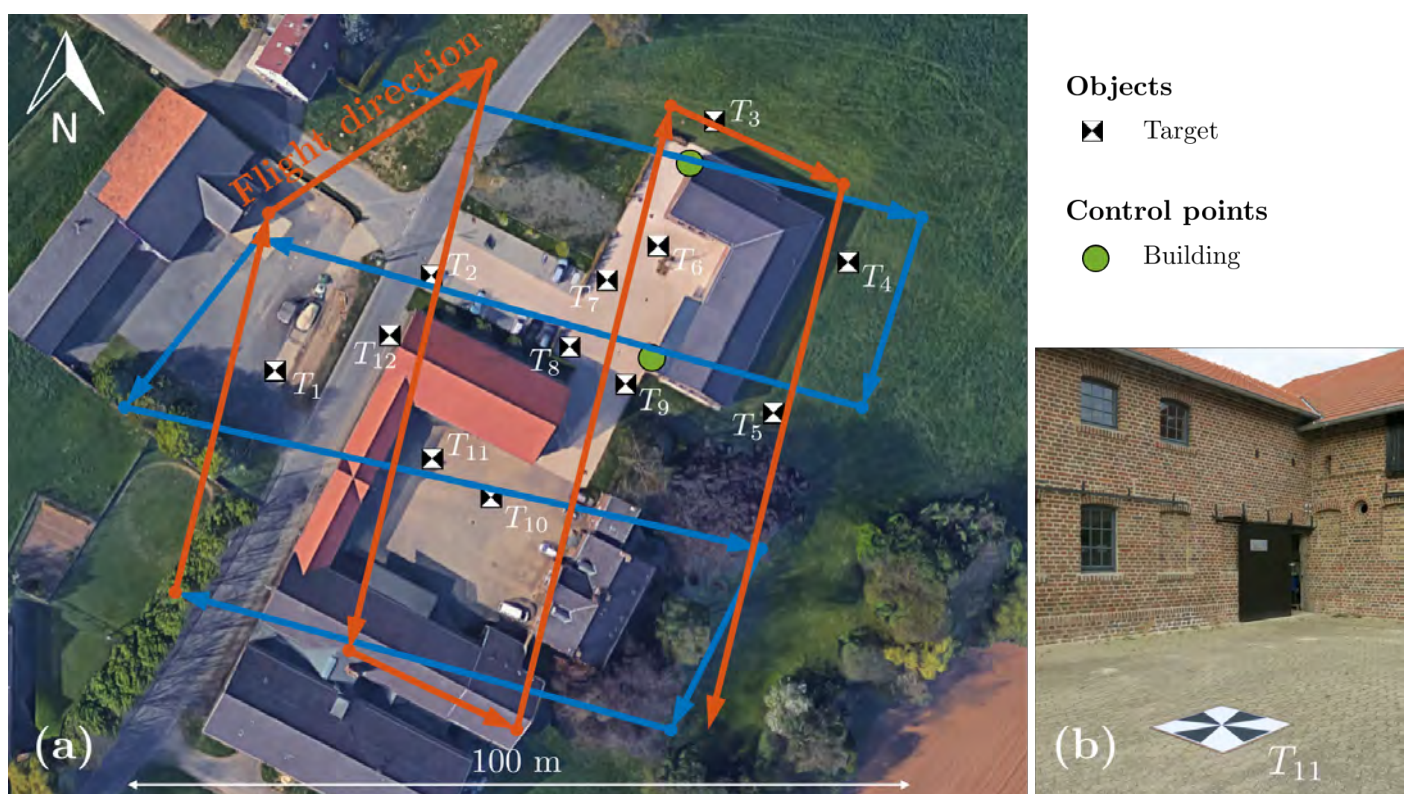
Figure 5. Second study area for the analysis of multiple strip measurement with included objects and the flight pattern of the individual measurement, © https://www.google.de/maps/ (accessed on 14 May 2021).
