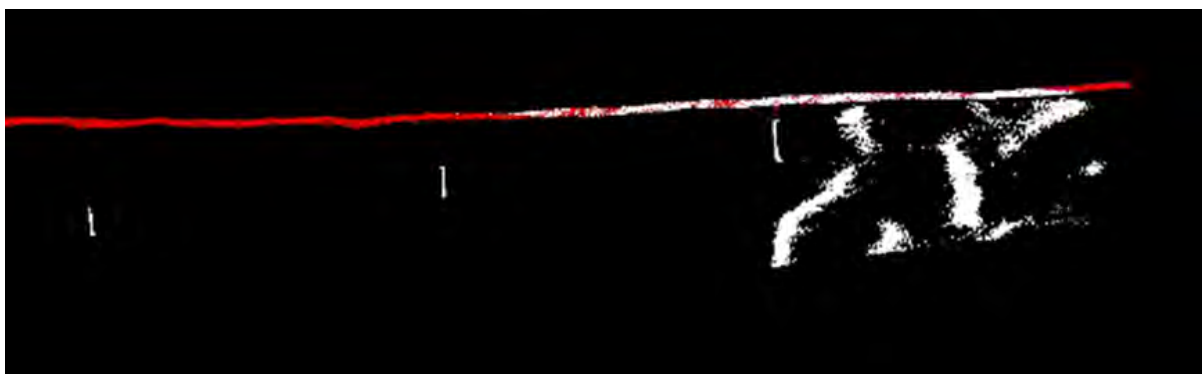
Figure 21: Laser scanner sees multiple echoes (dense smoke and laser targets behind, t=13:03:57 ).
