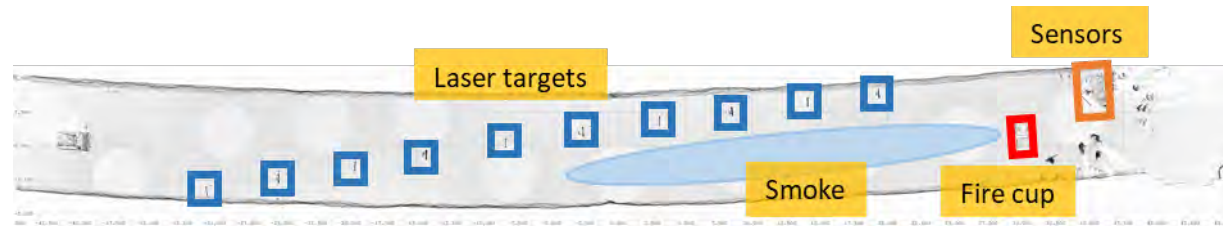
Figure 2: Floor plan of the test setup, point cloud of the composite laser scan (top view).
