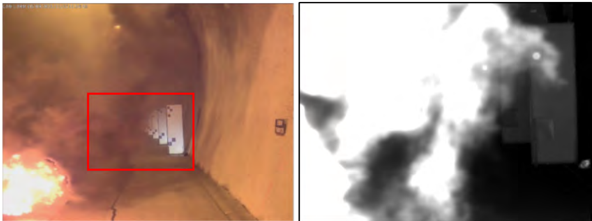
Figure 23: Glare of the thermal camera due to stinging flames or hot smoke in the foreground ( t=11:54:43 ).
