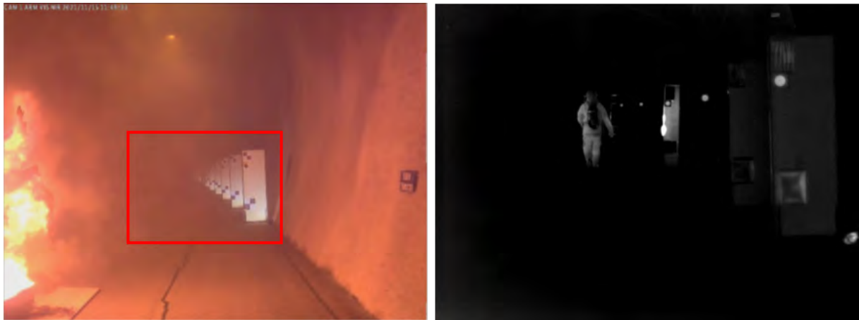
Figure 22: Comparison of a scene in the RGB and thermal image ( t=11:49:03 ).
