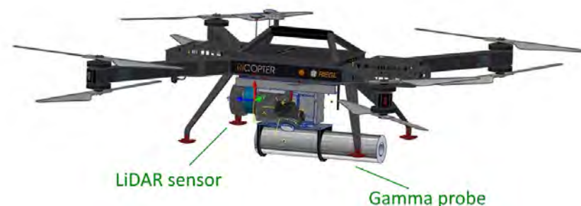
Figure 1. Carrier platform and sensor bundle comprising LiDAR sensor and gamma probe.
