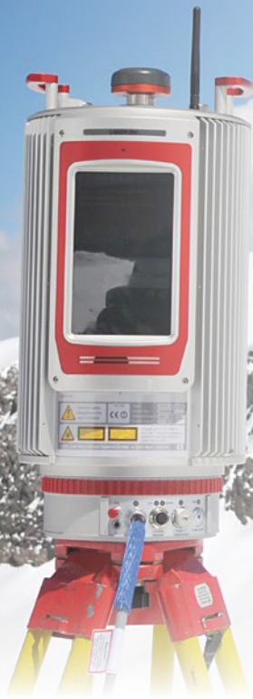
RIEGL VZ-6000 Terrestrial Laser Scanner for extremely long-range measurements up to 6,000 metres
