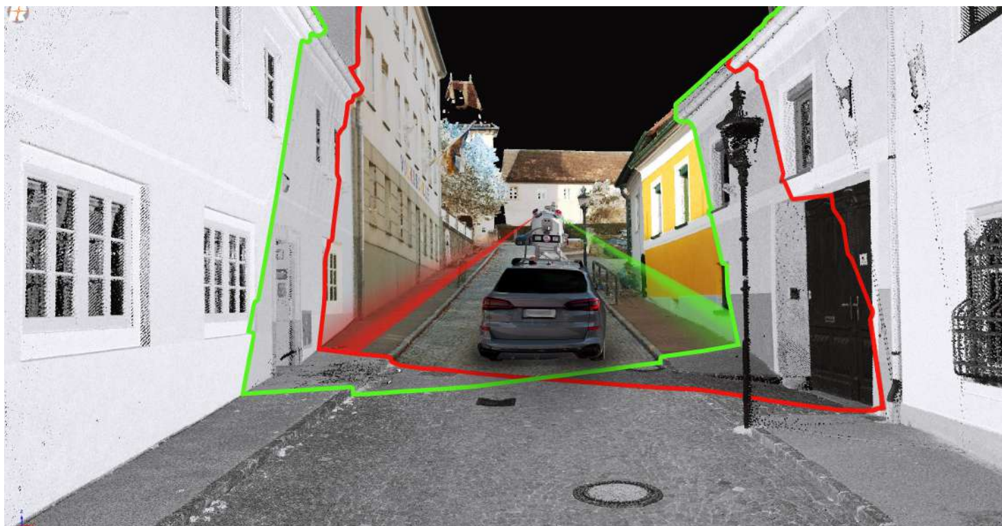
Figure 2: RIEGL VMX measurement principle: The image illustrates the "crossfire" scan lines of the two scanners (colored in red and green). The foreground shows the VMX point cloud colored with the reflectance attribute, the background shows the optional RGB colored point cloud.
