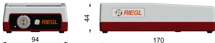
Fig. 1 Dimensional Drawing of the Dual Charger for RIEGL RBLI8S1P, all dimensions in mm
