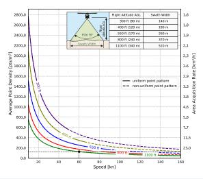
Example: VUX-240 $^{24}$  at 2,400,000 pulses/sec, laser power level 100% Altitude = 1,100 ft AGL, Speed 60 kn, resulting point density  $\sim$  125.93 pts/m $^2$
