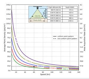
Example: VUX-240 $^{24}$  at 300,000 pulses/sec, laser power level 100% Altitude = 2,100 ft AGL, Speed 60 kn, resulting point density  $\sim 8.3$  pts/m<sup>2</sup>
