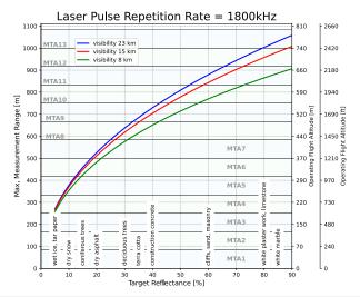
Operating Flight Altitude AGL given for the following conditions: FOV 75°, ambiguity resolved by multiple-time-around (MTA) processing, average ambient brightness, target size  $\geq$  laser footprint, roll angle  $\pm 5$
