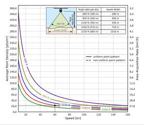
Example: VUX-240 $^{24}$  at 600,000 pulses/sec, laser power level 100% Altitude = 1,550 ft AGL, Speed 60 kn, resulting point density  $\sim 22.3$  pts/m $^2$
