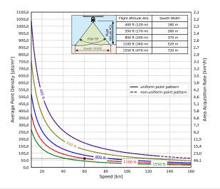
Example: VUX-240 $^{24}$  at 1,200,000 pulses/sec, laser power level 100% Altitude = 1,100 ft AGL, Speed 60 kn, resulting point density  $\sim$  63 pts/m $^2$
