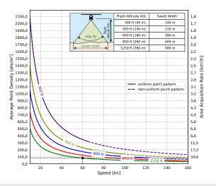
Example: VUX-240 $^{24}$  at 1,800,000 pulses/sec, laser power level 100% Altitude = 1,250 ft AGL, Speed 60 kn, resulting point density  $\sim$  83.1 pts/m<sup>2</sup>
